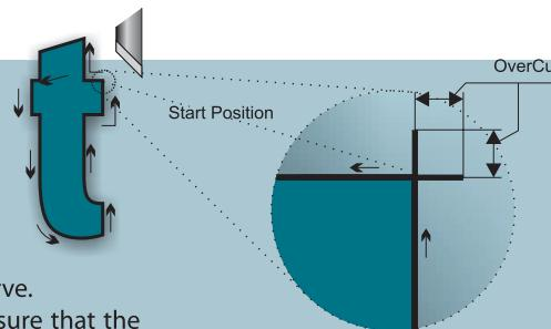
"OverCut" extends the vector in the beginning and at the end of a curve. This way it makes sure that the design is completely cut through. Without the "OverCut" function, due to a variety of tolerances, the cut line may not be completely closed causing difficulties when weeding.
