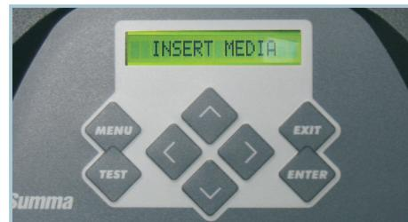
The large, easy-to-use control panel that allows you to quickly and easily change settings like speed, pressure and plot mode.
